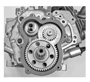
Step 3. Install the output gear (#4) to the output shaft (#3) and install the shaft/gear assembly into the housing making sure that the idler gear and the output gear mesh and line up properly. (Prior to installing the cover, take this opportunity to add 2.5 oz or 75cc of our Burris Gear oil in the gear case and on the bearings.) Prep the gasket (#12) with a light coating of WD 40 or light oil so it doesn't stick during disassembly and lay it on the gear housing/cover mating surface.
