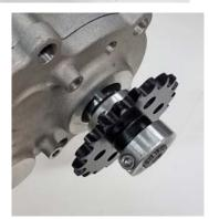
Step 4. Install the gearcase cover (#2) by sliding it over the output shaft being careful not to damage the shaft seal. In the process of sliding it over the crankshaft and idler shafts gently apply force from different sides to help keep them aligned. Be sure the cover is seating on the gasket and install the (#17) 7ea 14-20 Torx button head screws (T27 bit) and alternately
