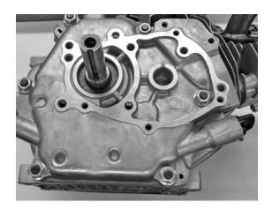
Step 1. Prep mounting surface and make sure the .75 dia crankshaft PTO is free of burrs and nicks and the gear and key are a sliding fit to accommodate assembly and disassembly. This is necessary on ALL shaft to bearing fits when assembling the gearbox! All machined mating surfaces require assembly lube or light grease during assembly.
