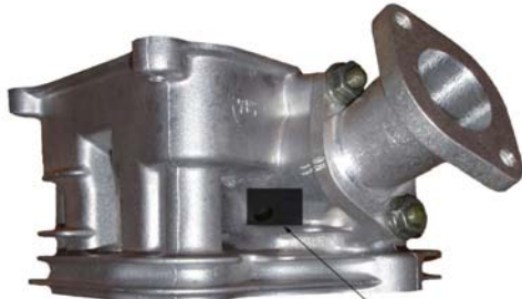
Approved Yamaha YF200 Inlet Tract Repair Area
